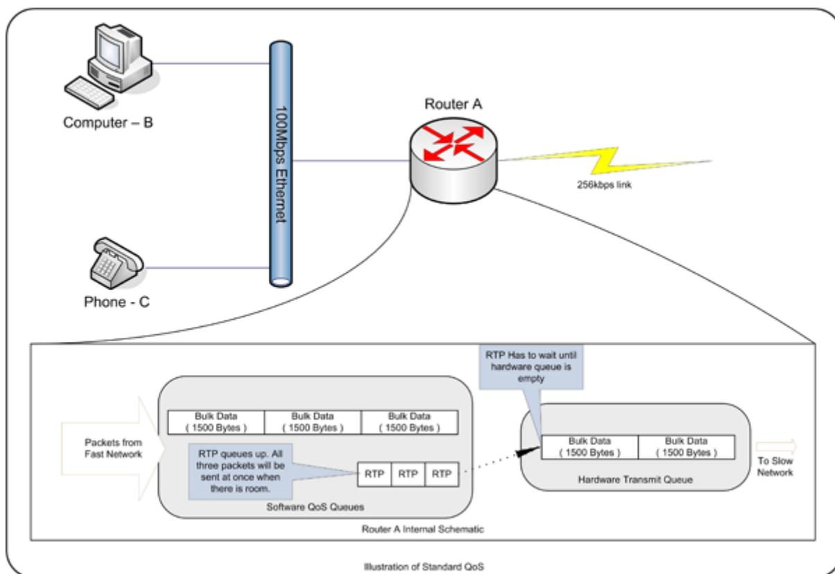
Data enters the router, A, from a 100Mbit/s LAN interface. A computer, B, on the LAN is sending an e-mail with a large attachment, and since the LAN is 100Mbit/s his computer sends many large ( typically 1500 byte ) packets to router A in quick succession. The router will continue to queue packets for sending to the WAN until its buffer fills up.
